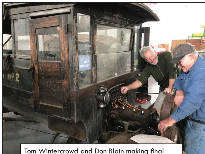
Tom Wintercrowd and Don Blain making final engine wiring adjustments.
