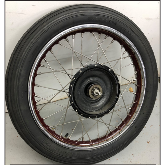
Turning the brake drum can be done without dismantling the wheel
