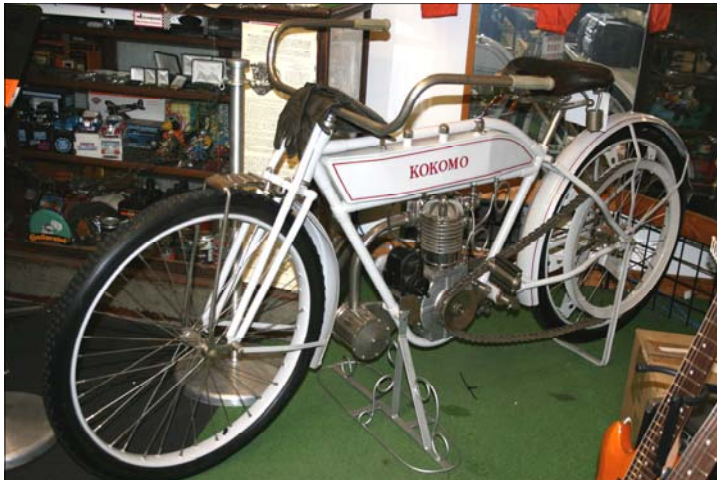
1911 Kokomo Motorcycle, 300cc side valve engine
